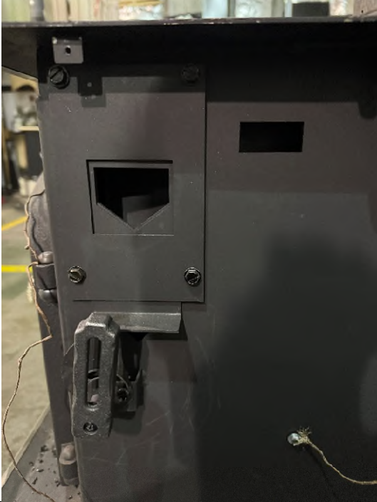
Air inlet minimum opening for minimum burn rate (Damper fully closed)
