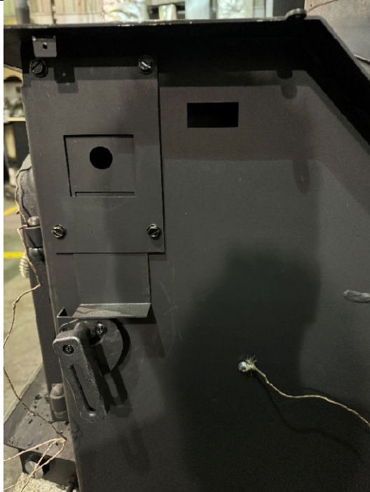
Air inlet minimum opening for minimum burn rate (Damper fully closed)
