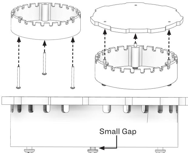
3. After assembling all the burner pieces, place it into the bottom of the firepit. Align the burner studs with the holes in the bottom of the firepit. Rotate the burner clockwise to lock into position. **NOTE: If a replacement Burner Kit (893653) is needed please call customer service.**
