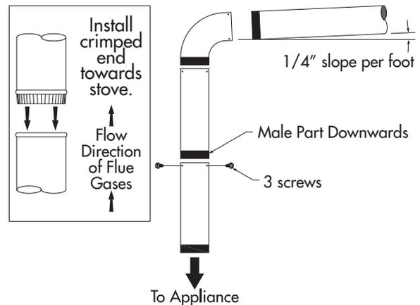
Your chimney connector and chimney must have the same diameter as the furnace outlet. If this is not the case, we recommend you contact your dealer in order to ensure there will be no problem with the draft.
