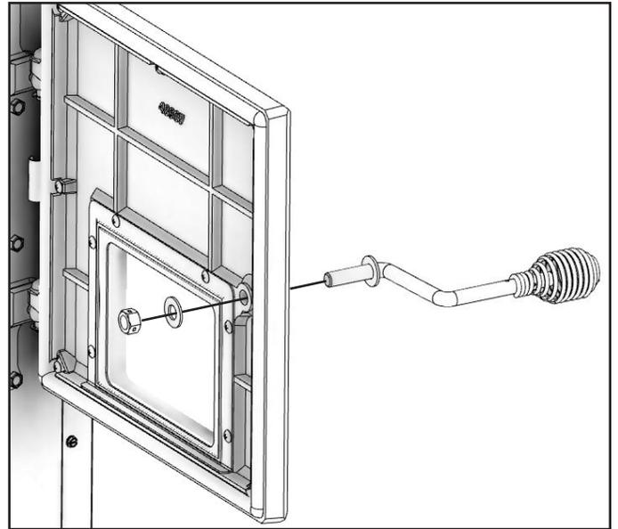
Use two (2) 1/4-20 x 3/4 bolts and two (2) washers to secure the latch assembly to the unit.
