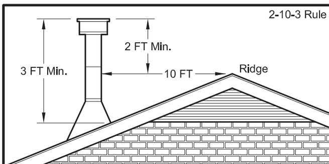
Your wood furnace may be hooked up with a factory built or masonry chimney, matching the diameter of the exhaust. If you are using a factory built chimney, it must comply with UL 103 or CSA-B365 standard; therefore it must be a Type HT (2100°F). It is extremely important that it be installed according to the manufacturer's specifications.
