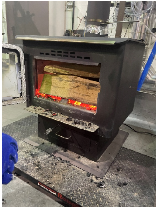
Low burn load in the firebox
