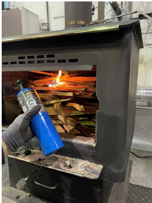
Startup and kindling ignition
