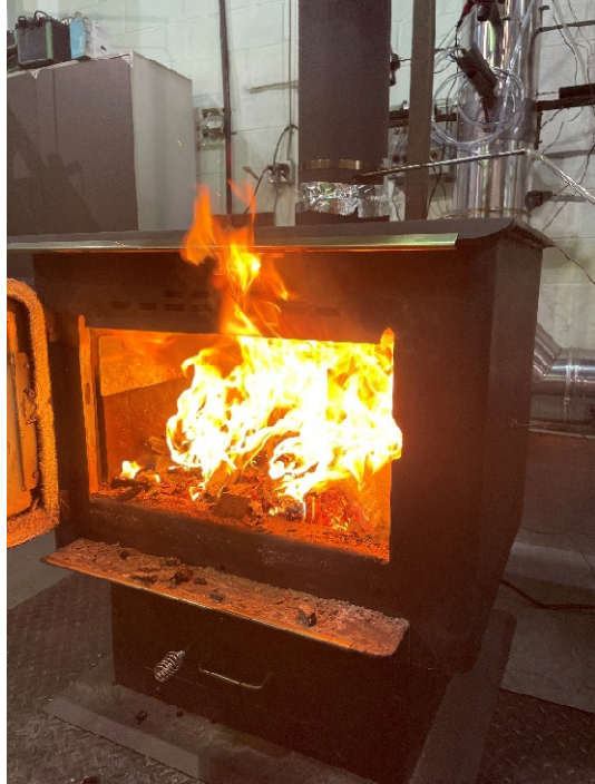
High burn load in the firebox
